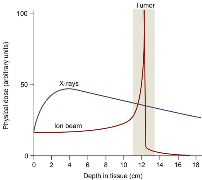
Fig. 1. Physical dose release along the path traveled in matter for X-ray and ion beam.
