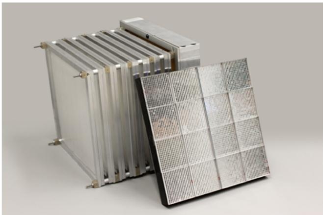
Fig. 2. Dose profiler. In foreground the calorimeter composed by  $64 \times 64$  matrix of pixelated LYSO crystals arranged in  $4 \times 4$  blocks, as described in Section 2.3. In background the 6 tracking planes of the tracker, as described in Section 2.1 and the plastic scintillator as described in Section 2.2.
