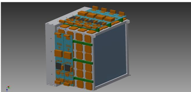
Fig. 3. The front-end electronics readout structure: in yellow the BASIC32\_ADC; in blue the FPGA controller (1 FPGA every BASIC32). (For interpretation of the references to color in this figure legend, the reader is referred to the web version of this article.)
