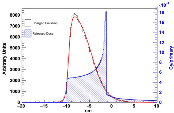
Fig. 5. Charged emission profile (red curve) and released dose (hatched figure) for a carbon ion beam impinging on a PMMA target from simulation.
