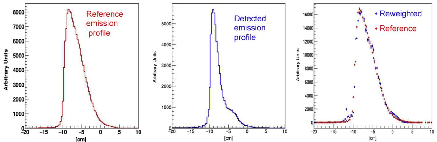
Fig. 7. Left panel: the MC profile of the emitted charged secondary as produced by the beam. Central panel: the emitted profile as reconstructed by the detector. Right panel: results of the re-weighting procedure.
