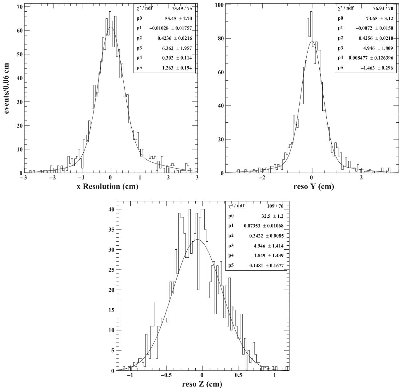
**Fig. 4.** Distribution of the difference between the measured and the true value of the proton origin coordinate  $x$  (beam direction),  $y$ ,  $z$  (profiler axes) for the full simulation (carbon ion beam coming along the  $x$  direction, at  $90^\circ$  with respect to the profiler axis and 2.5 cm radius of the target PMMA cylinder). Double Gaussian fits are superimposed to give an estimate of the corresponding resolutions.
